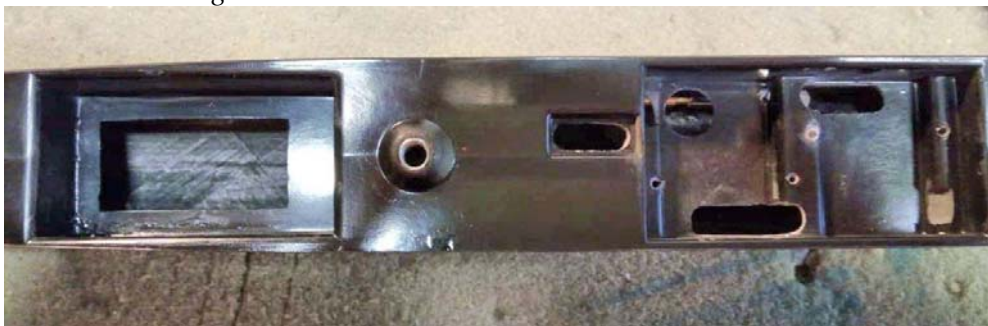
Cutting holes in fuse before assembly
